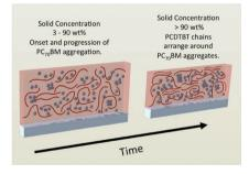
Thin-film formation in solution-cast PCDTBT:PC70BM 1:4 wt% blend films is characterised using a combination of spectroscopic ellipsometry and grazingincidence wide angle X-ray scattering. A multi-step process of structure evolution is observed which includes the coalescence of PC70BM molecules and an apparent delay in weak ordering within the PCDTBT-rich phases of the film.
