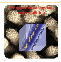
Hierarchical nanowire arrays based on a semiconductor core-layered double hydroxide shell are synthesized via a facile and cost-effective electrosynthesis method. The resulting core-shell ZnO@ LDH NW array exhibits largely enhanced efficiency in photoelectrochemical watersplitting, including a large photocurrent and high stability, as a result of the significantly improved photogenerated carrier transfer and increased reaction kinetics of water splitting.
