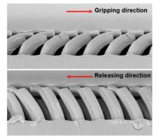
A switchable gecko-inspired adhesive that shows anisotropic adhesion and friction properties is presented. With proper actuation, the polymer-based dry adhesive provides strong adhesion and friction forces for attachment (or gripping), or weak forces for detachment (or releasing). The reusability of the dry adhesive is also demonstrated over multiple attachment/detachment cycles.
