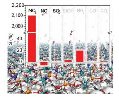
The tailored design of highly selective and sensitive gas sensors is the central issue in gas sensor technology. Density functional theory identifies the requirements for an efficient interaction between gas species and modified nanowires, enabling ultraselective detection. A prototype system with NO2 as the target gas shows extraordinary selectivity and sensitivity experimentally.
