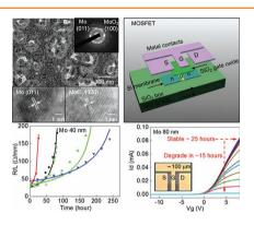
Effects of reactive dissolution on electrical conduction, morphological change, and chemical transformation of biodegradable metal thin films (Mg, Zn, W, Mo, and Fe) are studied for application of these metals in water-soluble transient electronic devices. Feasibility of using these dissolvable metals as contacts for n-channel silicon metal oxide field effect transistors (MOSFETs) is also demonstrated.
